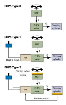
On loaders, large forklift trucks, dumpers, large tractors, combine harvesters, forestry machines and other heavy vehicles there is often need for electrically actuated steering in the form of a joystick or automatic steering. Electrically actuated steering acts as a supplement to hydraulic steering wheel control and facilitates optimised steering characteristics in different driving situations. In other words, it increases vehicle productivity and improves driving comfort.
